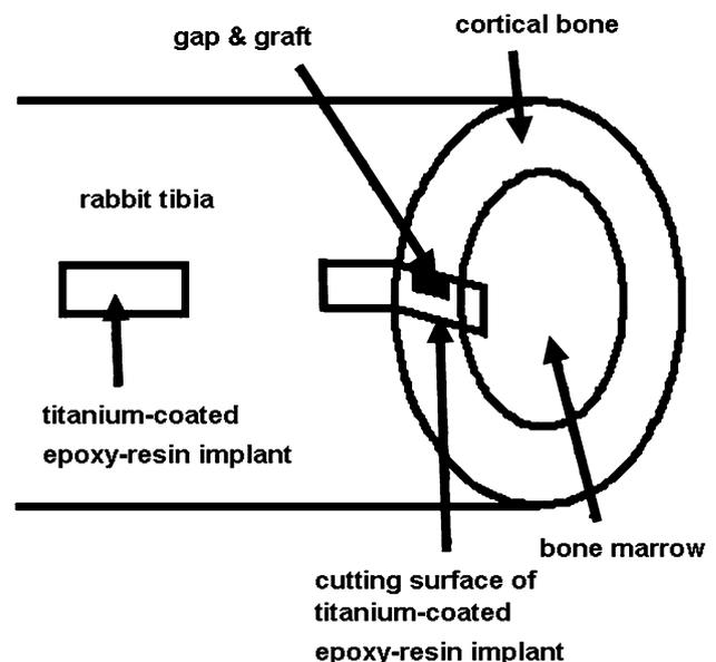
**Fig. 2** Schematic diagram of implantation of titanium-coated epoxy-resin block into tibia of rabbit. Three titanium-coated epoxy-resin block implants had different graft. (1) Control (no graft), (2) CAC, (3) DFDB, respectively. The gap size of titanium–bone interface was 0.5 mm in one subgroup and 1.0 mm in the other
