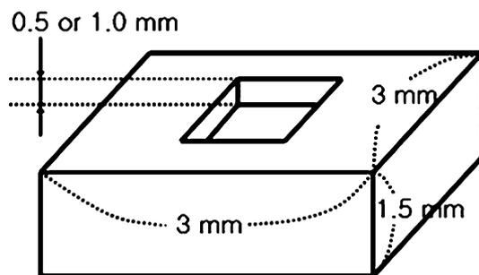
**Fig. 1** Titanium-coated epoxy-resin block implant. The surface was coated with pure titanium by use of ion sputtering coater. Each implant had a well of 0.5 or 1.0 mm depth
